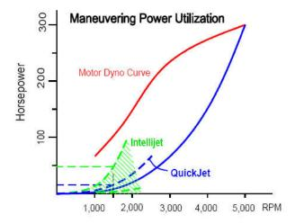
The hatched green area is the IntelliJet<sup>TM</sup>'s range of the continuously variable forward pitch in the maneuvering mode. This gives the operator a continuous range of forward thrust from full pitch to neutral. This continuous range extends into reverse thrust, where the operator also enjoys continuously variable thrust.
