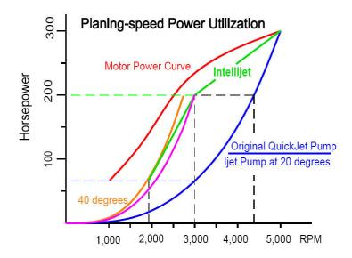
The blue curve on the right is the power demand curve on the original QuickJet and is also the power demand curve of the IntelliJet<sup>TM</sup> with the pump blades set to about 20 degrees. The orange curve is the power demand of the IntelliJet<sup>TM</sup> when the pump blades are set to about 40 degrees.
