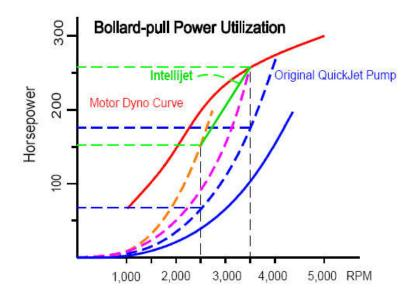
The dashed pump power curves indicate flow-restricted pump operation, which increases pump power demand and moderately reduces pump efficiency. The dashed blue curve is the power demand of the QuickJet pump at zero boat speed. The solid blue line is left in just to be consistent with the first graph, but it is not operative here.
