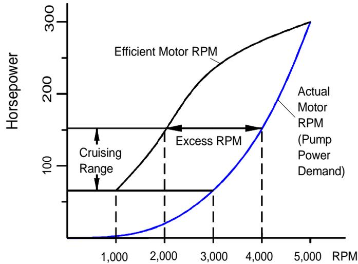
You can see that the motor must run at nearly twice its most efficient RPM to deliver power to the efficient pump. This results in 20% to 30% more fuel consumption. The more efficient total system again uses a less efficient pump that can provide continuously variable power transmission to operate the motor more efficiently. The following graphic shows the more efficient motor power demand curve resulting from this compromise.
