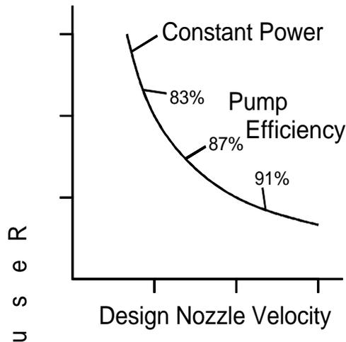
The resulting thrust force from a given amount of hydraulic power is the best measure of propulsion efficiency. It is clear from this that **the highest thrust force results from the design based on the lowest pump efficiency due to the much higher fluid power transfer efficiency.**
